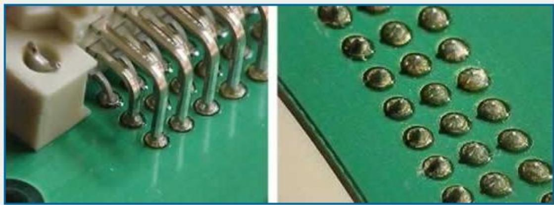
Views from both sides of a Pin-In-Hole-Reflowed connector
