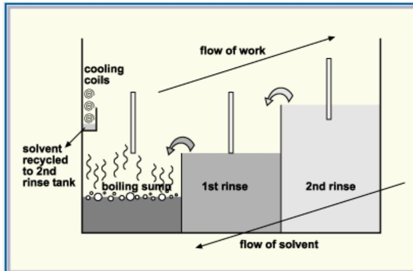
Figure 1: Schematic of a three-tank reflux cleaner as used for solvent cleaning processes
