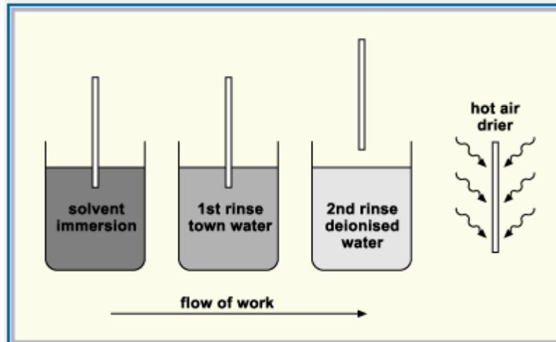
Figure 2: Schematic of a typical semi-aqueous cleaning process
