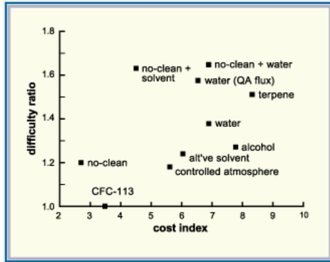
Figure 3: Difficulty:cost ratio for different cleaning methods
