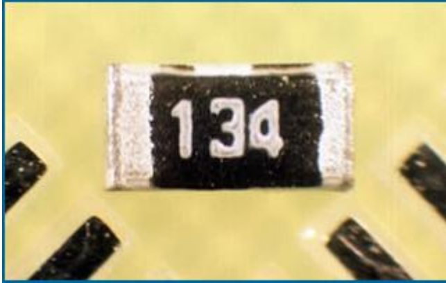
A completed and coded chip resistor
