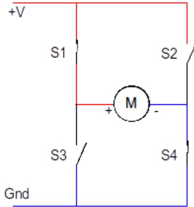
To change the direction switches S1 and S4 need to be opened and then S2 and S3 closed. The positive supply is now provided to the right of the motor and the negative to the left, so the motor will now turn in the opposite direction.
