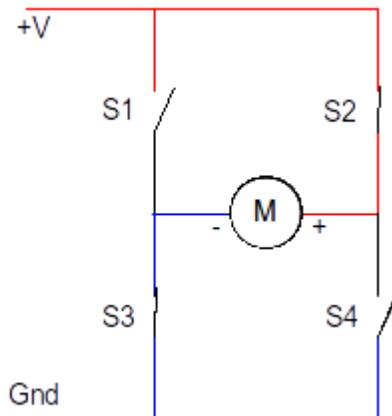
**It is important that S1 and S3 are never closed at the same time and the same with S2 and S4. Switching these on together would create a short circuit across the power supply.**
