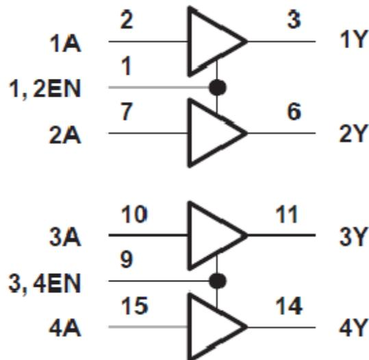
To check that the IC is suitable we should refer to the datasheet available from the manufacturer (in this case Texas Instruments). According to the datasheet the IC can be used to switch up to 1A for supplies of 4.5V to 36V, and includes a separate power supply for the input to output. All inputs are compatible with TTL and CMOS logic, which will work with both the GPIO from the Raspberry Pi and the Arduino. The power supply for the IC needs to be 5v which is the same as the Raspberry Pi.
