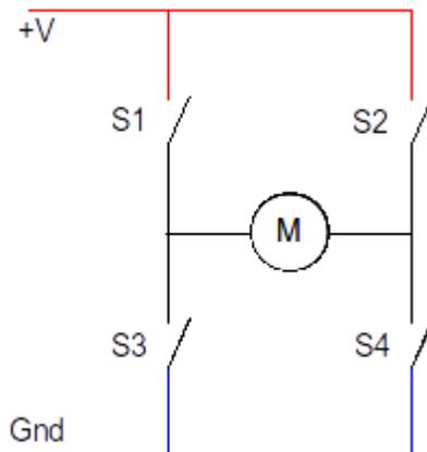
When S1 and S4 are closed the positive supply goes to the left of the motor and the negative to the right. The motor will then work in one direction.
