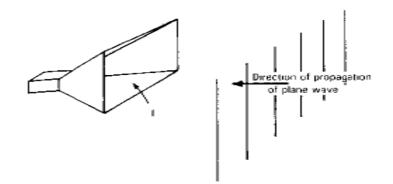
Let the poynting vector or power density of the plane wave be S watts/sq -m and let the area or physical aperture be  $A_p$  sq-m. If the Horn extracts all the power from the Wave over it's entire physical Aperture  $A_p$ , Power absorbed is given by  $P=SA_p=(E^2/Z)A_p$  Watts, S is poynting vector,
