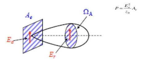
Assuming a uniform field E<sub>r</sub> in far field at a distance r, Power Radiated is
