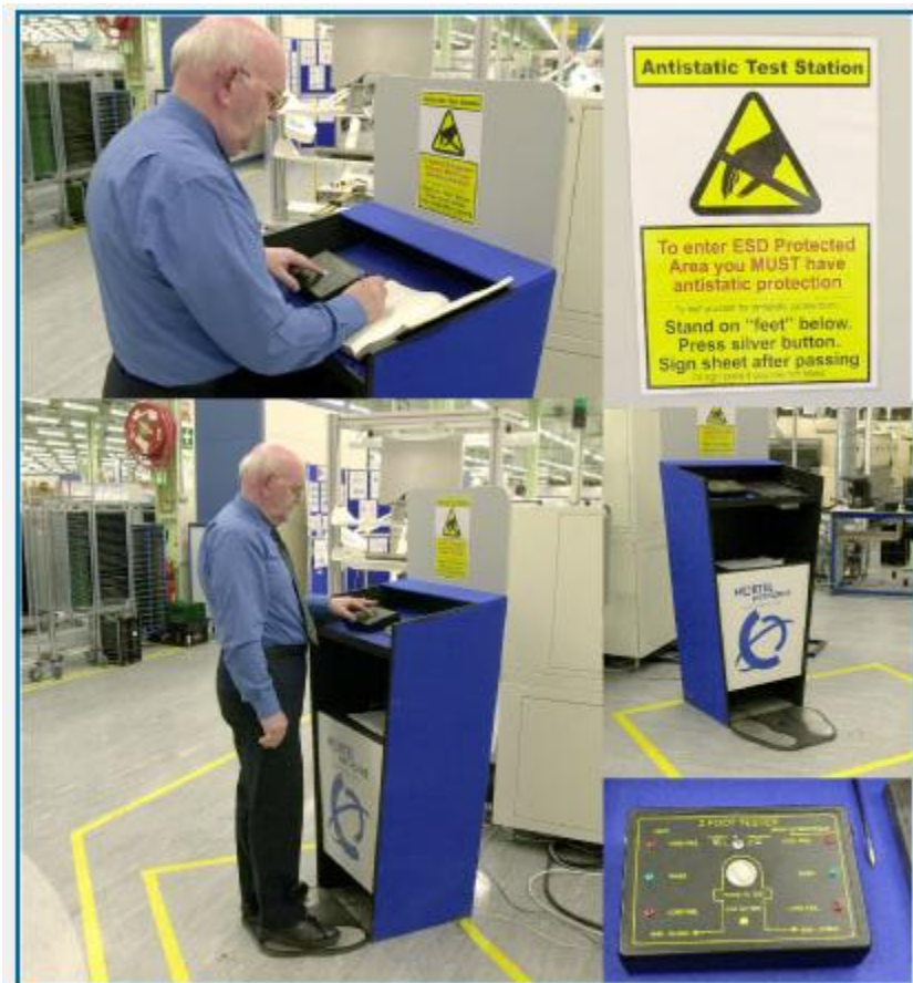
Figure 2: Checking personal grounding for effectiveness
