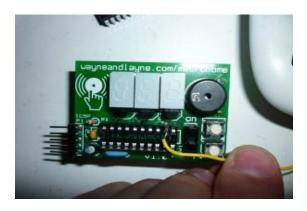
Place a tiny loop of wire in pin 12's spot. You can also see where I cut the trace above pin 12.
