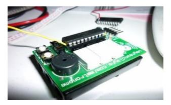
Push the chip back down, trapping the wire loop.
