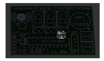
The PCB trace to cut, just above pin 12. Click to enlarge.
