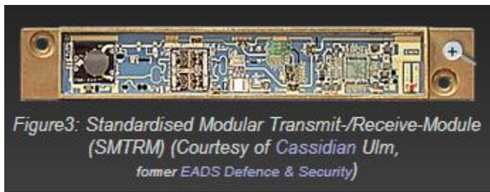
Figure3: Standardised Modular Transmit-/Receive-Module (SMTRM) (Courtesy of Cassidian Ulm, former EADS Defence & Security)
