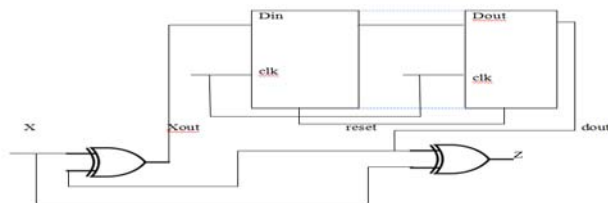
Fig 4 Control circuit having D flip-flops and XOR gates
