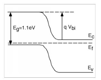
Figure 3: Band diagram for a p-n junction
