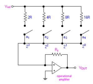
The binary inputs, ai (where i = 1, 2, 3 and 4) have values of either 0 or 1. The value, 0, represents an open switch while 1 represents a closed switch.
