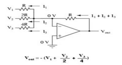
The circuit for a 4-bit DAC using binary weighted resistor network is shown below:
