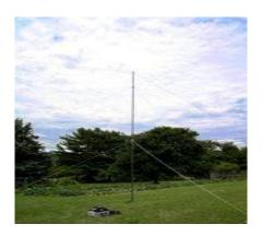
I have wanted to build a multi-band wire antenna for some time now and this past Field Day I had an opportunity to use a very good one. The Carolina Windom is essentially an off-center fed dipole (OCFD) that uses a portion of its feed line as a vertical radiator. I used one to make about a 100 PSK31 contacts on 20, 40, and 80 meters during Field Day.
