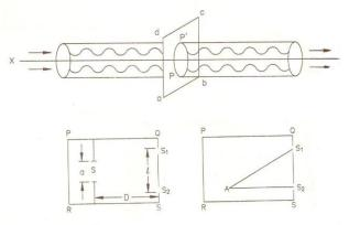
The beam is said to possess spatial coherence if the phase difference of the waves crossing P and P' at any instant remains constant
