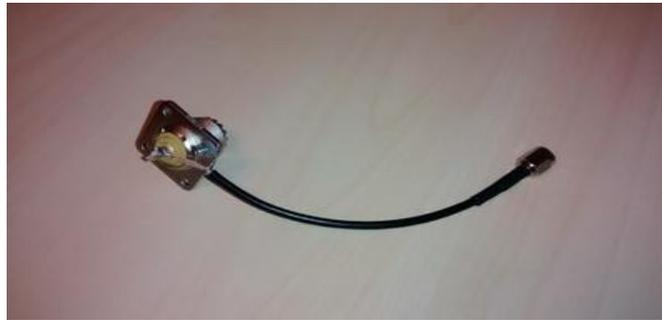
Lately I have been preparing a handful of new receivers for deployment. The way you're supposed to wire a panel-mounted SO-239 (left on the picture above) to an internal coaxial cable was another reminder that this setup was not made with high frequency signals in mind.
