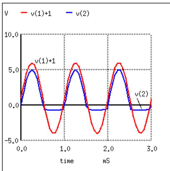
$V(1)+1$  is actually  $V(1)$ , a 10 V<sub>ptp</sub> sinewave, offset by 1 V for display clarity.  $V(2)$  output is clipped at -0.7 V, by diode D1.
