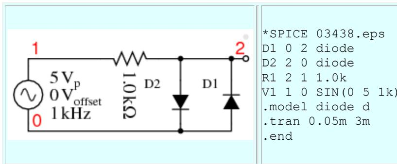
*Symmetrical clipper: Anti-parallel diodes clip both positive and negative peak, leaving a  $\pm 0.7$  V output.*
