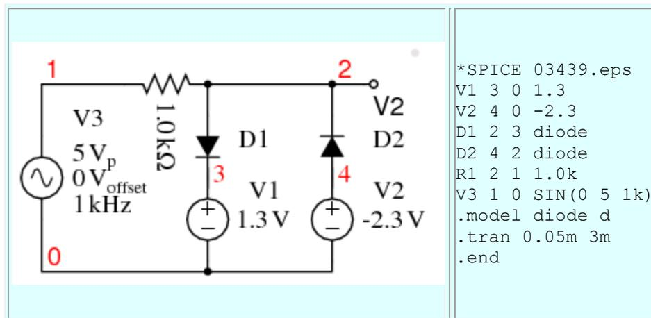
D1 clips the input sinewave at  $2\text{ V}$ . D2 clips at  $-3\text{ V}$ .
