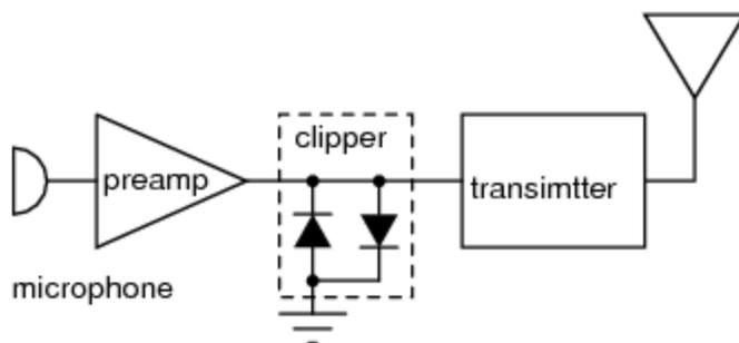
*Clipper prevents over driving radio transmitter by voice peaks.*
