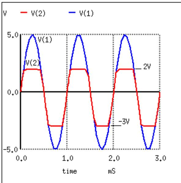
*D1 clips the sinewave at 2V. D2 clips at -3V.*
