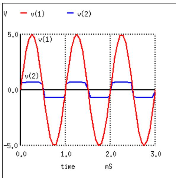
Diode D1 clips at  $-0.7\text{ V}$  as it conducts during negative peaks. D2 conducts for positive peaks, clipping at  $0.7\text{ V}$ .
