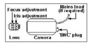
Some very wide angle lenses do not have a focus ring. The 'BNC' plug is used for connecting the coaxial video cable. Line powered cameras do not have the mains cable there power is provided via the coaxial cables.
