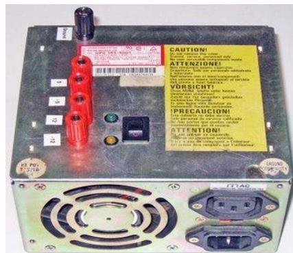
The newly born power supply will turn off nicely when you short its outputs or when the load exceeds its maximum power output capacity (i.e. when you plug a big motor or a power tool to it). By combining the outputs (DC) you can get 5V (GND to 5V), 7V (5V to 12V), 10V (-5V to 5V), 12V (GND to 12V), 17V (-5V to 12V), and 24V (-12V to 12V).
