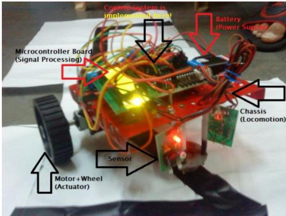
Basic Parts of a Robot – All the parts mentioned above are marked
