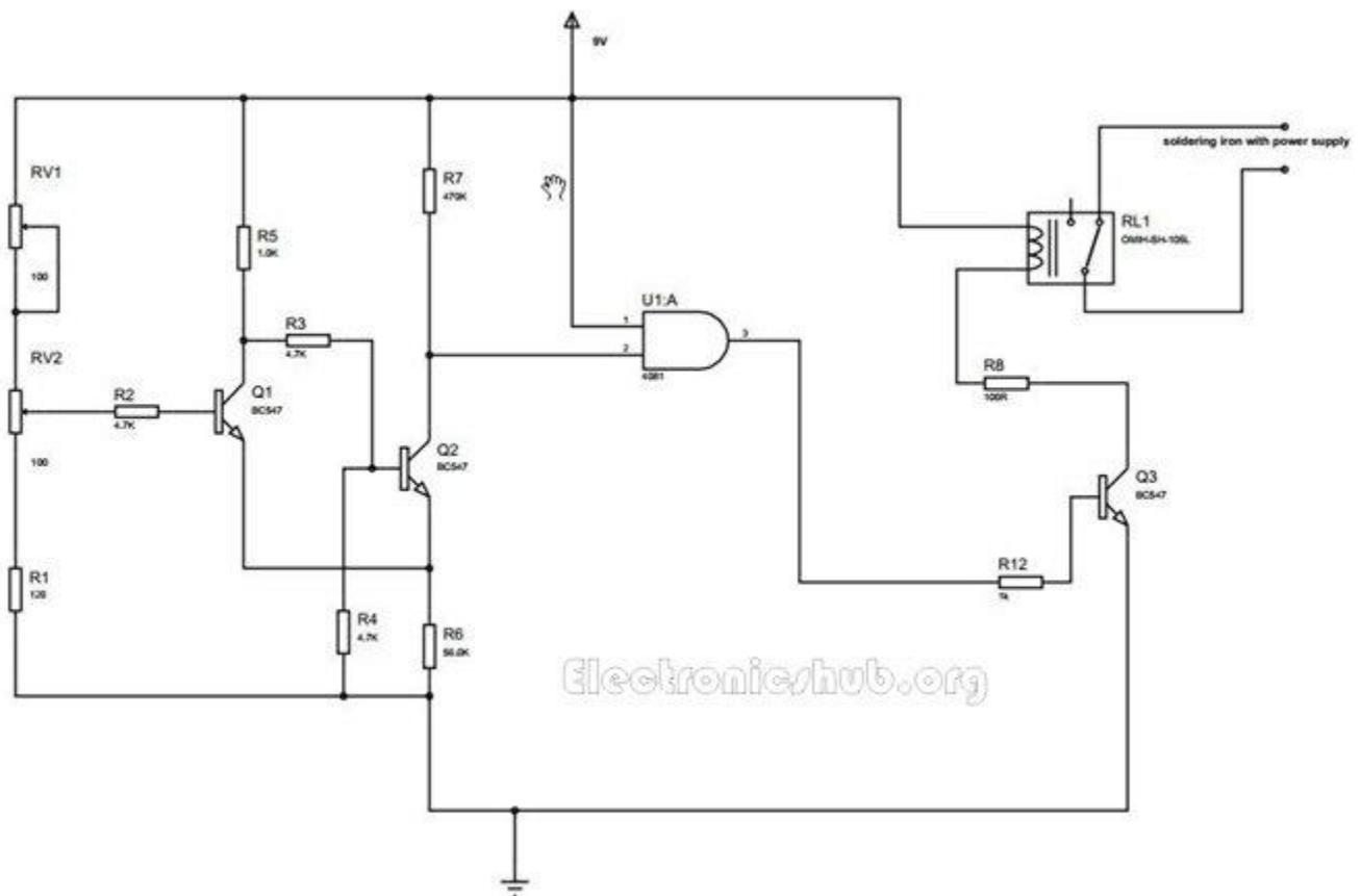
The circuit uses a thermistor for detecting the temperature of the circuit. The resistance of the thermistor is inversely proportional to the temperature thereby the temperature of the thermistor decreases with increase of temperature and its resistance increases with decrease of temperature. This means that the thermistor is a temperature sensitive device with negative coefficient of temperature. Negative coefficient of temperature
