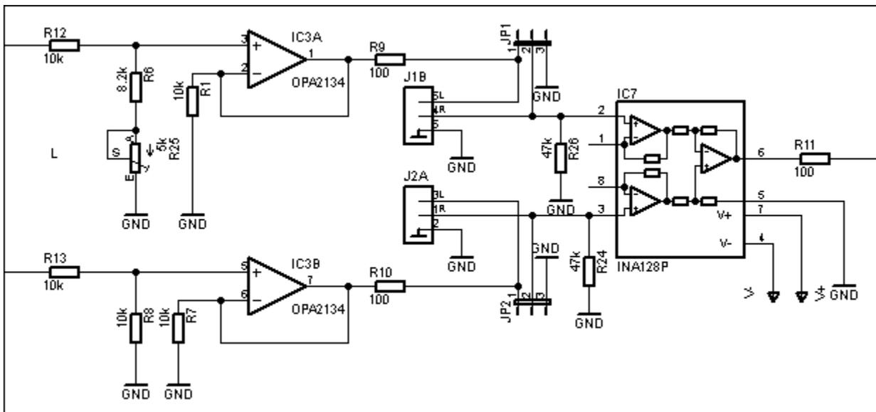
Figure 1. One channel of the difference amplifier.
