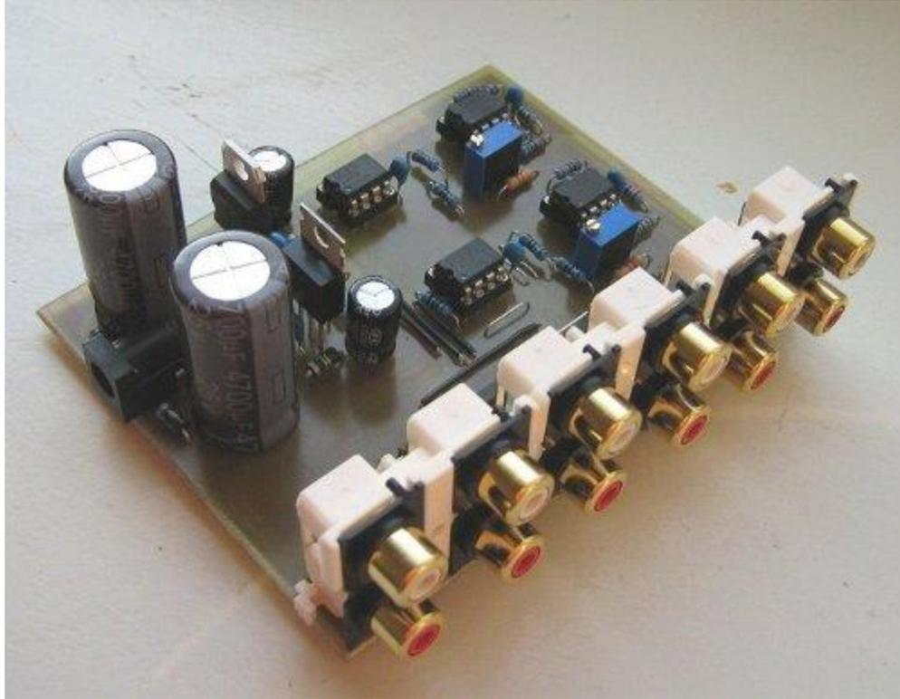
Figure 2. Constructed version of the difference amplifier.
