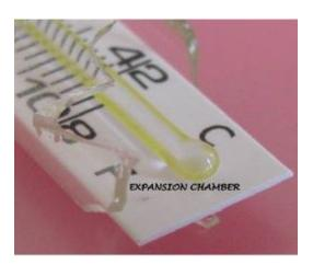
The top most part of the capillary tube is called the Expansion Chamber. It is hemispherical in shape to provide more space for the gases to expand. When the mercury rises with the increase in temperature in the tube, the gas or air present in the chamber moves upward in the expansion chamber. This space is also utilized by the
