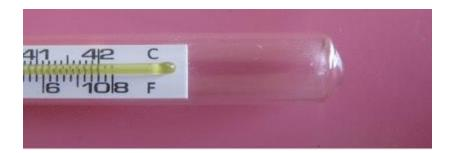
The Glass Chamber is the top most part of the Thermometer called protection chamber. It is used to protect the whole body of thermometer containing capillary tube, scale and mercury from coming in contact with the outside world.
