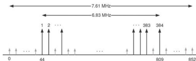
Fig. 1. The P1 symbol in the DVB-T2 system
