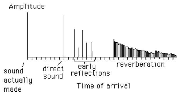
**Fig. 4 Time and amplitude of sounds at listener's ear**
