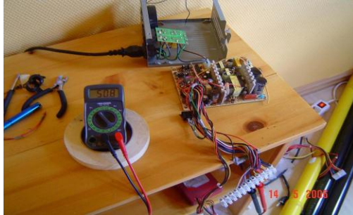
50.8 volts from the +12V and -12V rails combined.
