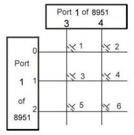
Keyboard circuit of the Robotic car
