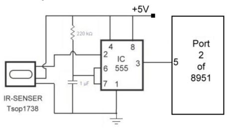
Circuit diagram of IR Receiver
