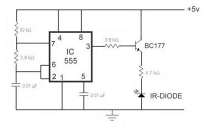
Circuit diagram of IR Transmitter
