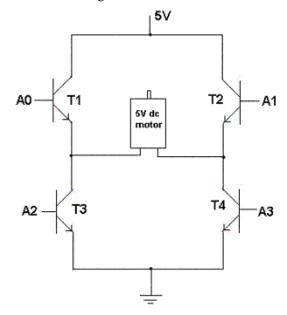
Circuit diagram of Motor connection
