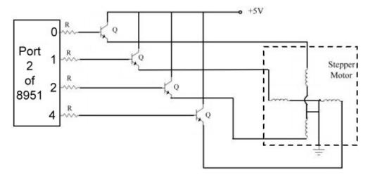
Interfacing stepper motor to 8951
