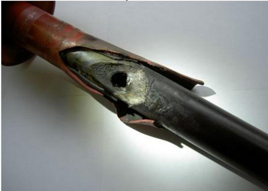
Damaged electrical cable due to the partial discharge (photo by JIM CAHILL at emersonprocessxperts.com)
