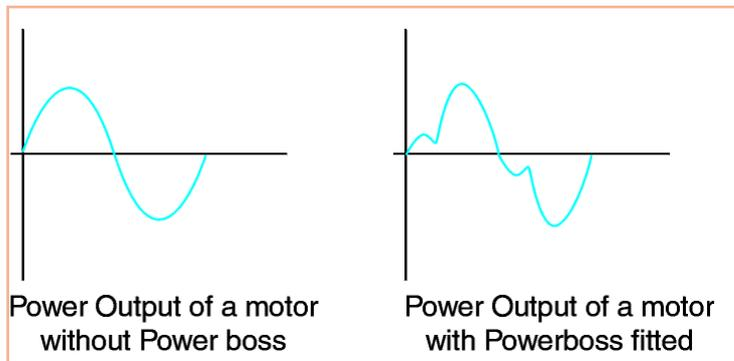
(rpm) due to momentum. But it does have a reduction in voltage and current, which is power. Figure 5 shows a typical example of a sinewave before and after the PowerBoss principle has been applied. The shape of the graphs are not accurate due to every motor having its own characteristics.
