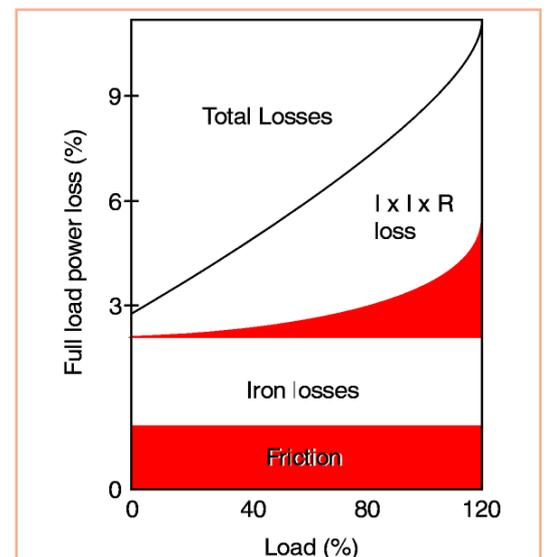
Figure 1. Graph of power losses in electric motors
