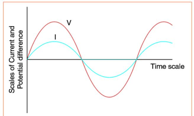
Figure 2. V and I are in phase for a purely resistive load.
