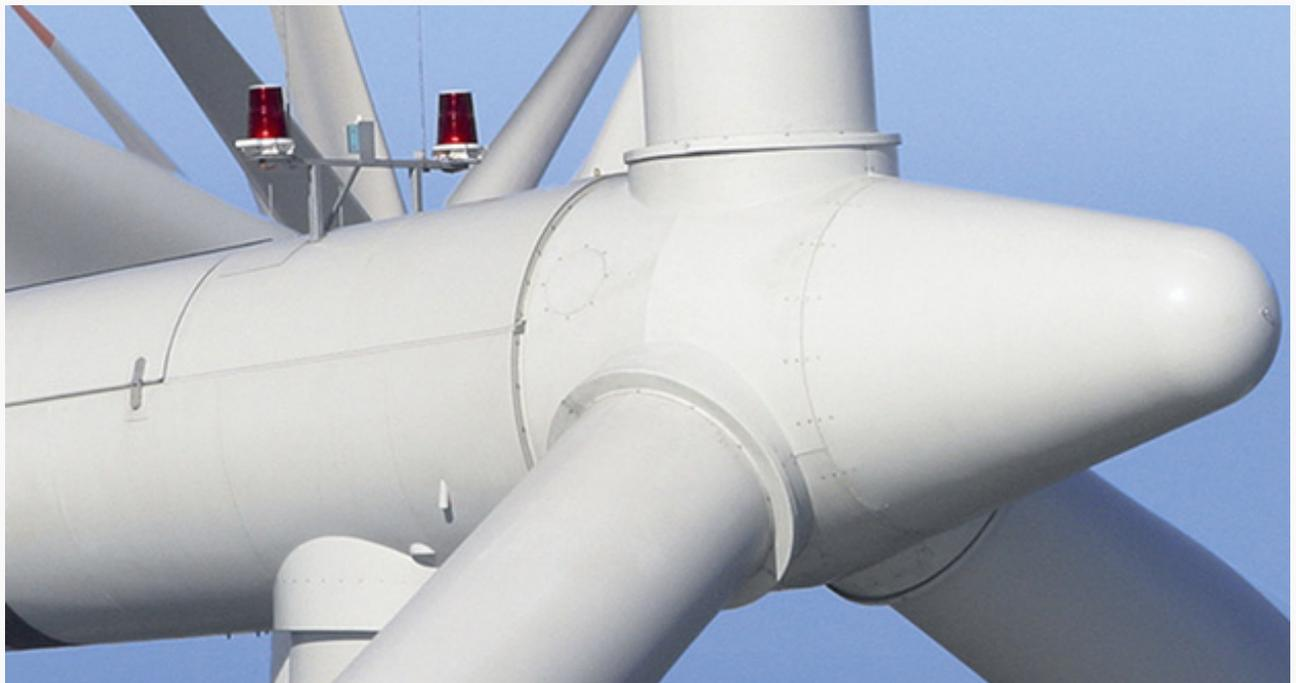
Wind turbine lighting signalization (on photo: SIEMENS wind turbine)
