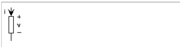
**Figure 1:** The generic circuit element.
