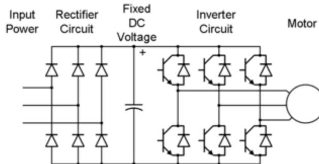
When an induction motor is connected to a full voltage supply, it draws several times (up to about 6 times) its rated current. As the load accelerates, the available torque usually drops a little and then rises to a peak while the current remains very high until the motor approaches full speed.
