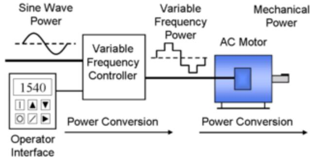
An embedded microprocessor governs the overall operation of the VFD controller. The operator interface, also commonly known as an Human Machine Interface (HMI), provides a means for an operator to start and stop the motor and adjust the operating
