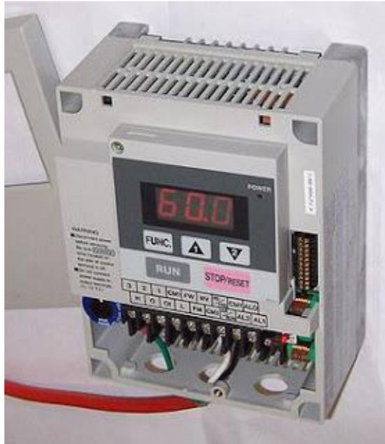
Variable-frequency drives are also known as adjustable-frequency drives (AFD), variable-speed drives (VSD), AC drives, micro-drives or inverter drives. Since the voltage is varied along with frequency, these are sometimes also called VVVF (variable voltage variable frequency) drives.
