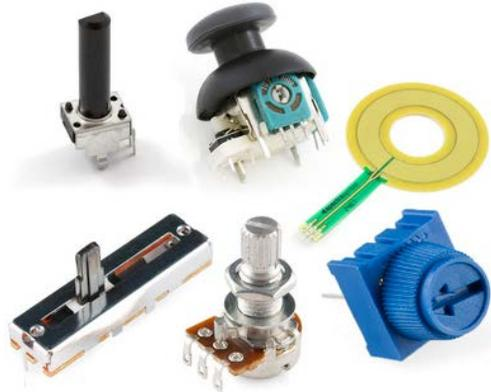
*A smattering of potentiometers. From top-left, clockwise: a standard 10k trimpot, 2-axis joystick, softpot, slide pot, classic right-angle, and a breadboard friendly 10k trimpot.*
