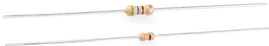
*A half-watt ( $\frac{1}{2}W$ ) resistor (above) sized up to a quarter-watt ( $\frac{1}{4}W$ ).*
