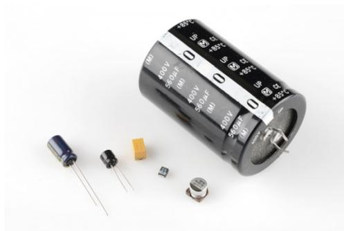
*An assortment of through-hole and surface-mount electrolytic capacitors. Notice each has some method for marking the cathode (negative lead).*
