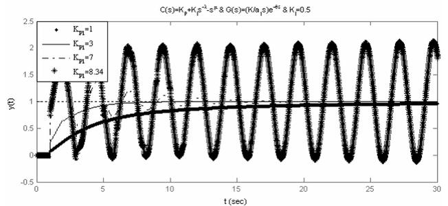
Fig. 8 Step responses for first order time delay system with using lead compensator
