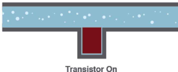
Likewise, under the right circumstances, a transistor can look like a **short circuit** between the collector and emitter pins. Current is free to flow through the collector, and out the emitter.
