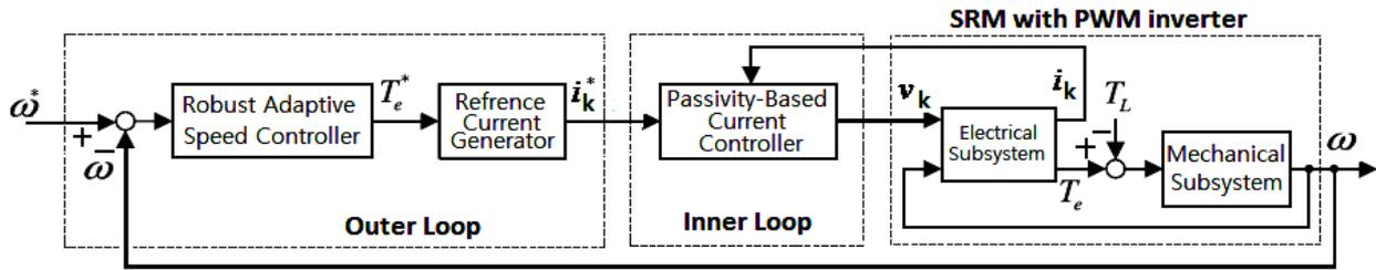
Fig. 3 Block diagram of the overall speed control system
