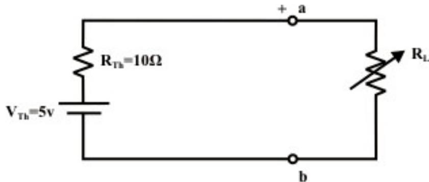
The choice of  $R_L$  that absorbs maximum power from the circuit is equal to the value of Thevenin resistance  $R_{Th}$
