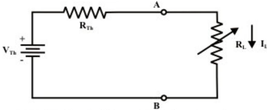
**Fig. 8.6(b): The circuit for maximum Power transfer**
