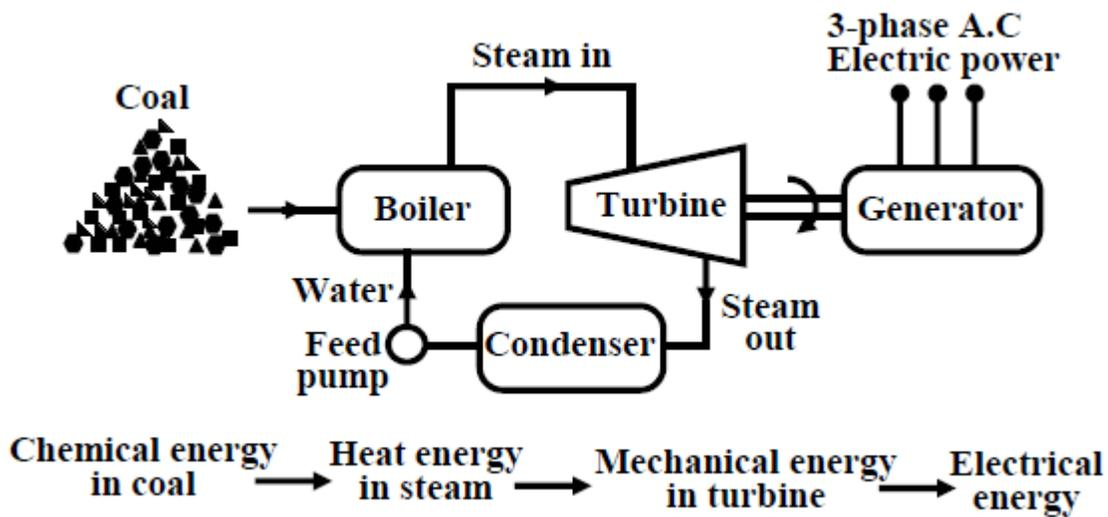
Figure 2.1: Basic components of a thermal generating unit.
