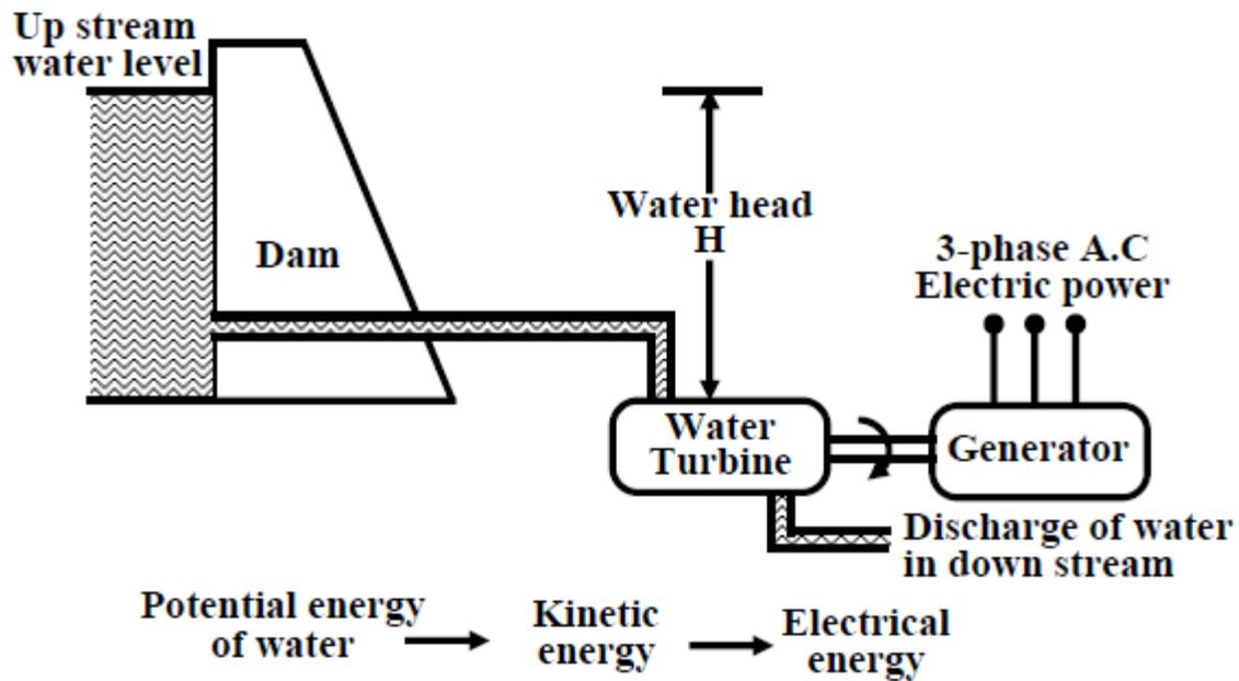
Figure 2.2: Basic components of a hydal generating unit.
