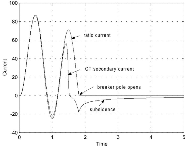
**Figure 5** Subsidence current from a CT output after the breaker poles open
