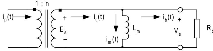
$i_p(t)$  = primary current [A]                       $V_s$  = CT secondary voltage output [V]
