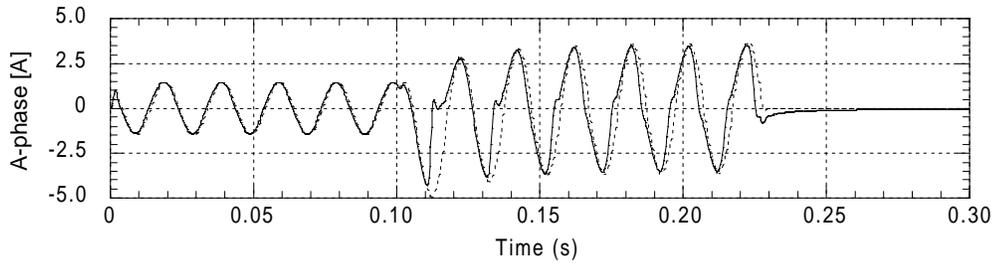
**Figure 2** Saturated (solid) and normal (dashed) currents
