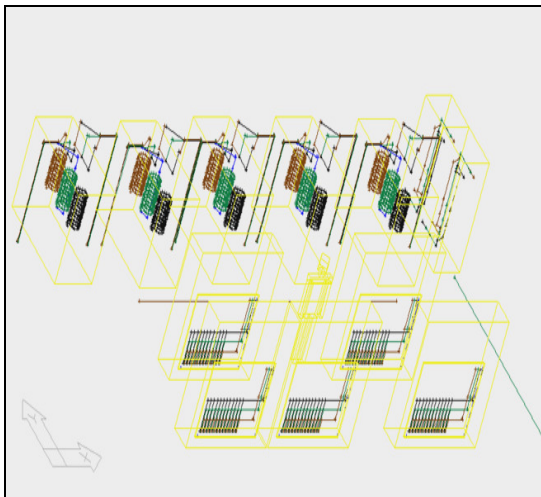
Fig. 7 3D presentation of disposition TS 2 20/0.4 kV in EFC-400 software
