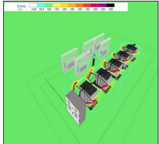
Fig. 8 Distribution of electrical field intensity TS 2 20/0.4 kV – 2D continual distribution
