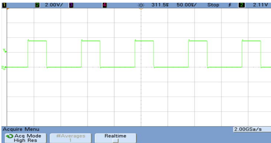
Fig. 12 PWM pulse in sensorless control
