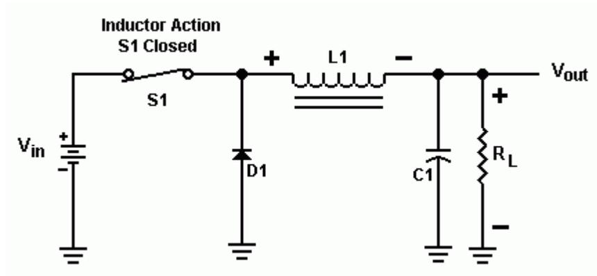
As we see above, L1, which tends to oppose the rising current, begins to generate an electromagnetic field in its core. Notice that diode D1 is reverse biased and is essentially
