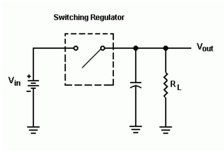
The time that the switch remains closed during each switch cycle is varied to maintain a constant output voltage. Notice that the primary filter capacitor is on the output of the regulator and not the input. As is apparent, the switching regulator is much more efficient than the linear regulator achieving efficiencies as high as 80% to 95% in some circuits. The obvious result is smaller heat sinks, less heat and smaller overall size of the power supply.
