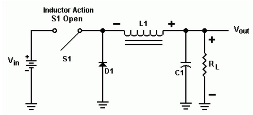
As we see in this diagram the electromagnetic field that was built up in  $L1$  is now discharging and generating a current in the reverse polarity. As a result,  $D1$  is now conducting and will continue until the field in  $L1$  is diminished. This action is similar to the charging and discharging of capacitor  $C1$ . The use of this inductor/diode combination gives us even more efficiency and augments the filtering of  $C1$ .
