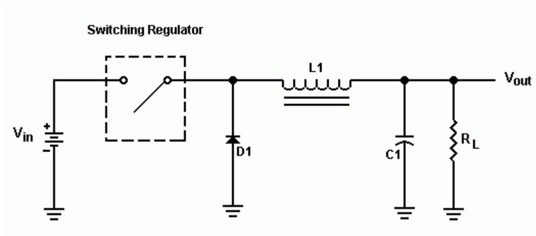
As we see above the switching regulator appears to have a few more components than a linear regulator. Diode D1 and Inductor L1 play a very specific role in this circuit and are found in almost every switching regulator. First, diode D1 has to be a Schottky or other very fast switching diode. A 1N4001 just won't switch fast enough in this circuit. Inductor L1 must be a type of core that does not saturate under high currents. Capacitor C1 is normally a low ESR (Equivalent Series Resistance) type.
