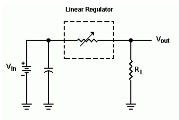
The primary filter capacitor is placed on the input to the regulator to help filter out the 60 cycle ripple. The linear regulator does an excellent job but not without cost. For example, if the output voltage is 12 volts and the input voltage is 24 volts then we must drop 12 volts across the regulator. At output currents of 10 amps this translates into 120 watts (12 volts
