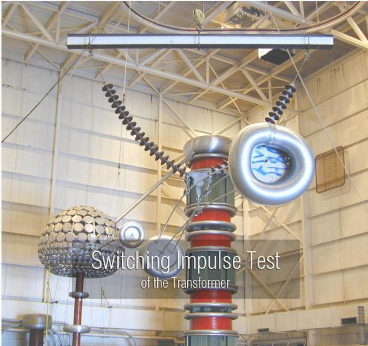
*Switching Impulse Test of the Transformer (on photo Mississippi State University High Voltage Laboratory as University Research Center)*
