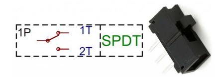
An SPDT switch circuit symbol, and an <u>SPDT slide switch</u>.
