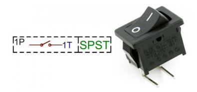
The circuit symbol for an SPST switch in the off position and a <u>through-hole, right-angle,</u> <u>maintained, SPST, rocker switch</u>.
