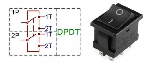
A DPDT circuit symbol, and a 6-terminal <u>DPDT rocker switch</u>.
