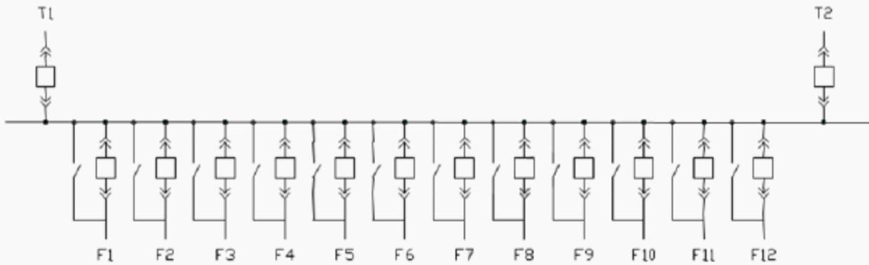
Figure 2: Single Bus scheme with Bypass Isolator
