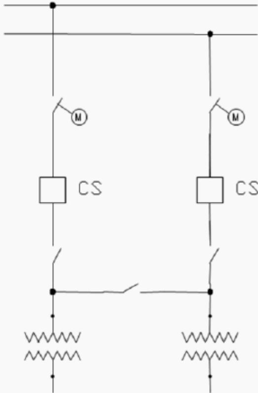
Figure 10: Double feed Scheme
