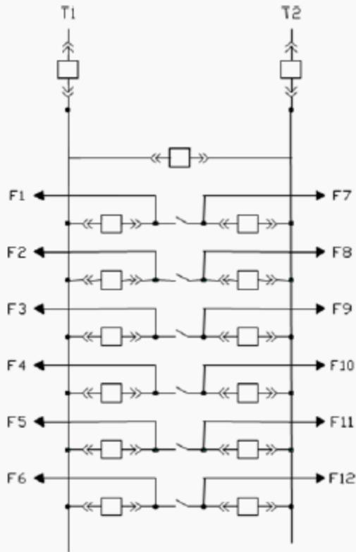
Figure 3: Single Bus scheme with Bypass Switch between Two adjacent Bays
