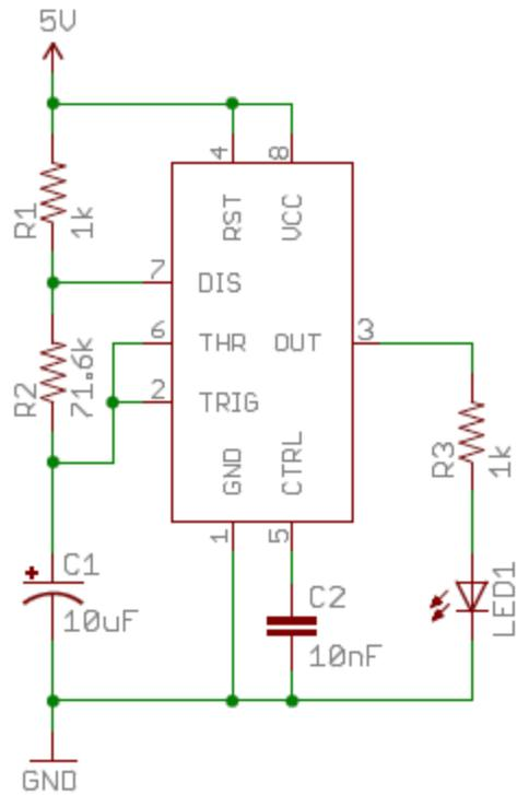
*In this circuit, resistors play a key role in setting the frequency of the 555 timer's output. Another resistor (R3) limits the current through an LED.*
