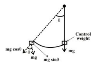
At equilibrium i.e. for steady deflection, Deflecting torque = Controlling torque. If the instrument is gravity controlled
