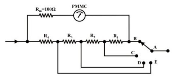
Fig. 42.12: An Ayrton shunt has several services connected shunts in parallel with PMMC.
