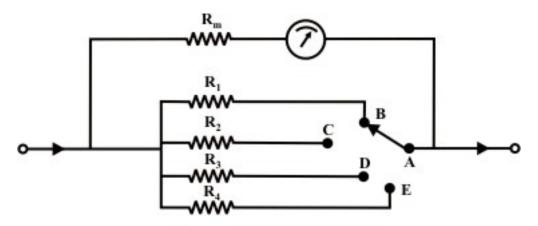
Fig. 42.2(b): Multi-range ammeter circuit
