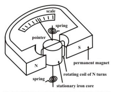
Fig. 42.1(a): Permanent Magnet Moving Coil Instrument.
