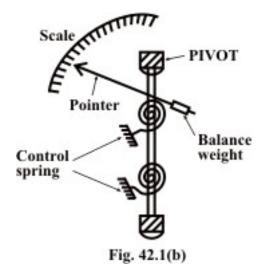
Fig. 42.1(a) shows the basic construction of a PMMC instrument. A moving coil instrument consists basically of a permanent magnet to provide a magnetic field and a small lightweight coil is wound on a rectangular soft iron core that is free to rotate around
