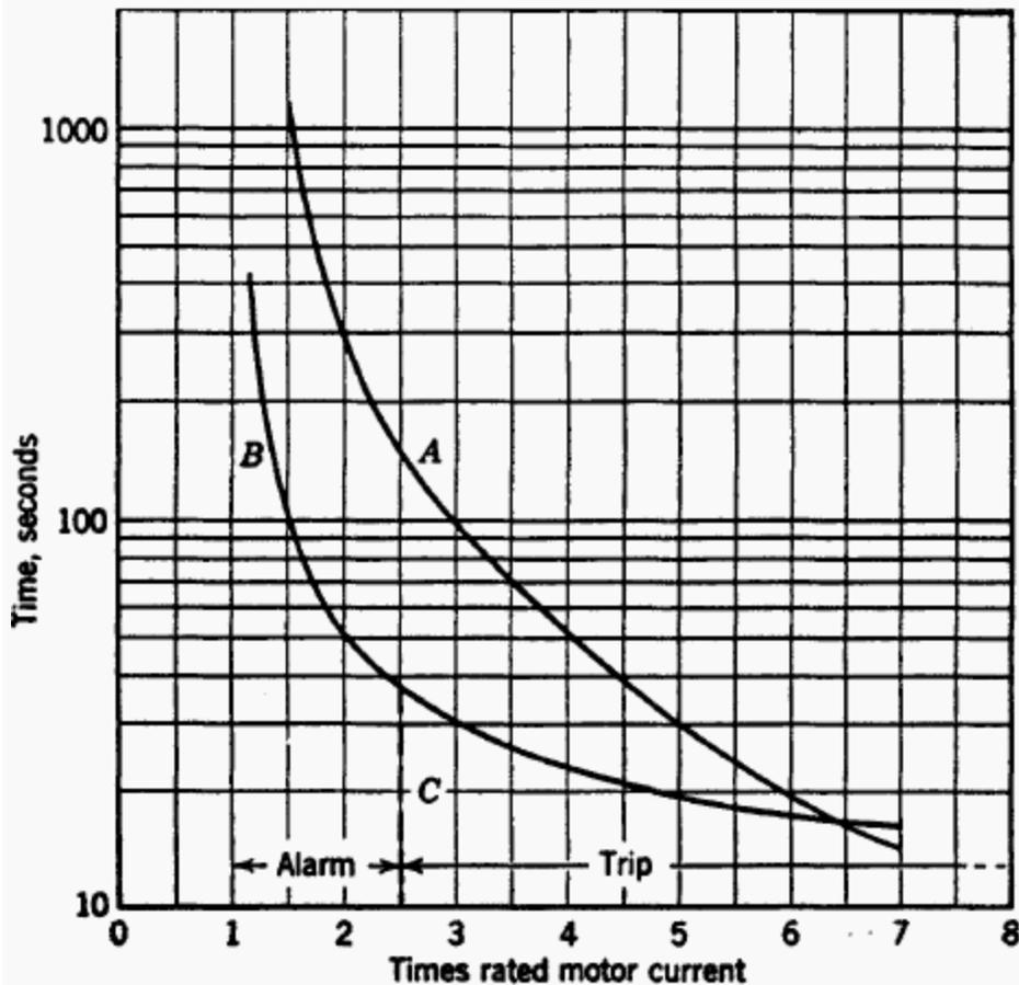
Figure 3 - Protection characteristic for essential-service motors. A, motor; B, inverse-time relay; C, instanteneous relay.
