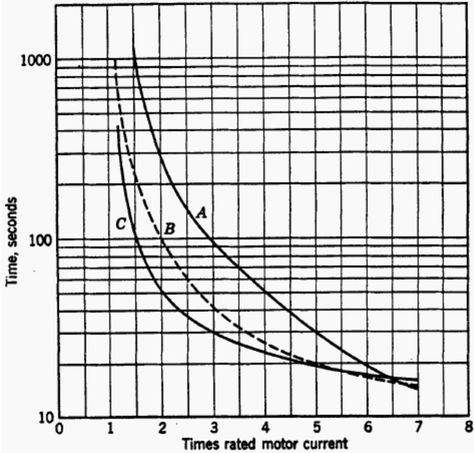
Figure 2 - Typical motor-heating and protective-relay characteristics. A, motor; B, replica relay; C, inverse-time relay.
