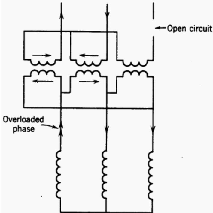
Figure 1 - Illustrating the need for overcurrent protection in each phase
