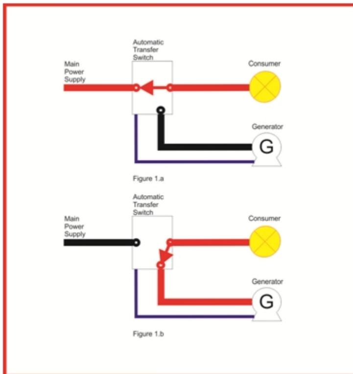
In figure 1 the red lines indicates the presence of power, the black lines indicate the absence of power and the blue line is the startup line of the generator. We can see in 1.a the main power supply line has power and is connected to the consumer and in 1.b the absence of power in the main supply line has triggered the Automatic Transfer Switch to connect the consumer to the Generator.
