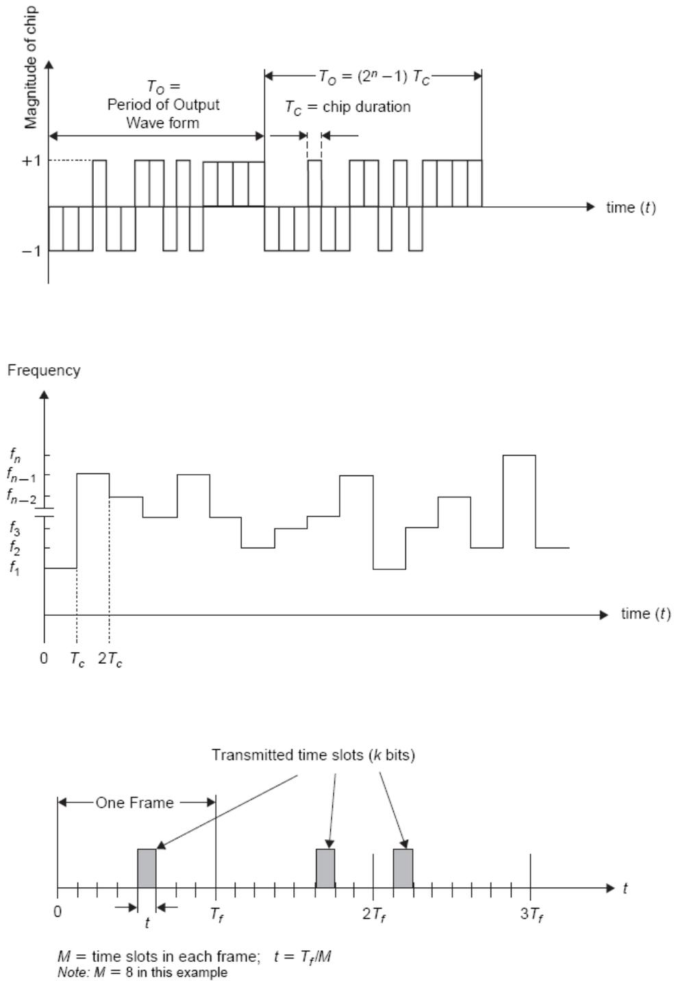
**Figure 11.1 Spread spectrum techniques.**
