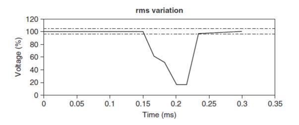
Figure 2.4 (a) Voltage sag due to a single line-to-ground fault
