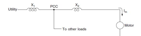
Figure 2.4 (b) Circuit that can exhibit voltage sag due to motor starting
