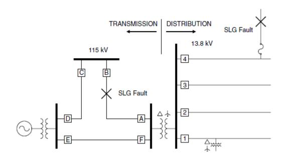
Figure 2.3 Fault locations on the utility power system
