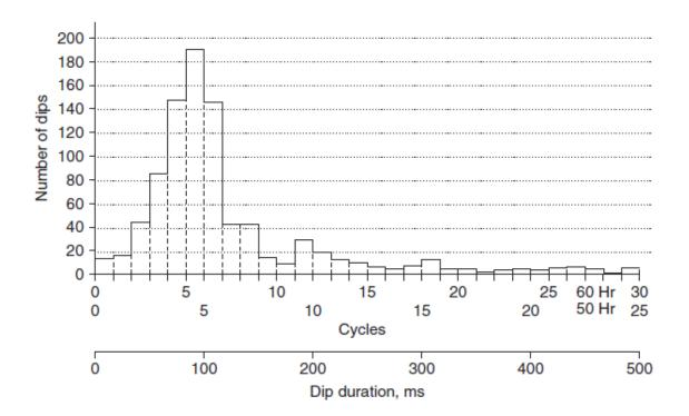
Figure 2.4(d) Histogram of voltage sag duration from EPRI study on voltage dips in U.S.Systems
